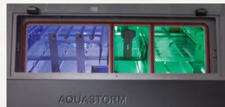
AS FSM with wash pump upgrade with mixed spray technology and chemical isolation as shown.
